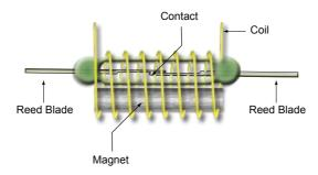
Not surprisingly normally closed relays are more difficult to manufacture and have higher magnetic interaction due to the bias magnet.
