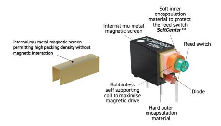
The magnetic shield is made of Mu metal which has a high permeability at low frequencies and DC. It deflects any external magnetic field around the relay body and the material has a low ability to retain a magnetic field when the coil current is interrupted. Magnetic shields using other materials are generally to be avoided since remanent magnetism can alter the operating point of the relay and create contact variability.
