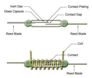
Different reed switches require different levels of magnetic field to close the contact, and this is usually quoted in terms of the ampere turns (AT) – simply the product of the current flowing in the coil multiplied by the number of turns. Again this creates a great deal of variation in the reed relay characteristics. Stiffer reed switches for higher power levels or high voltage switches with larger contact gaps, usually require higher AT numbers to operate, so the coils require more power.
