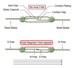
If a magnetic field is applied along the axis of the reed blades the field is intensified in the reed blades because of their ferromagnetic nature, the open contacts of the reed blades are attracted to each other and the blades deflect to close the gap. With enough applied field the blades make contact and electrical contact is made.
