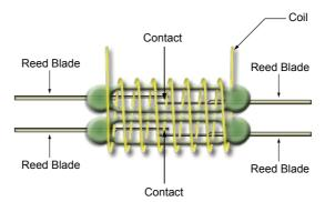
It is important to remember that these relays do not have an interlock mechanism between the two, it is unsafe to assume that that the two poles operate at exactly the same time and the two reed switches are essentially independent. There could be an operate time difference of between 50 - 250 microSeconds between them. Failure in one (say a contact weld) will not stop the other contact from moving.
